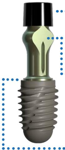
Plastic cap prevents impression material from entering access hole. It remains in the impression when post is removed, which provides a firm seat for the coping after curing.
