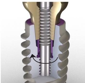
Continue to turn the abutment removal tool until the abutment releases from the tapered connection of the implant.
