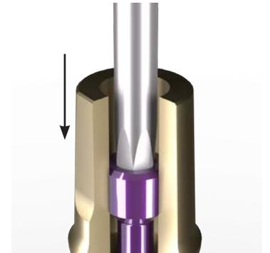
Apply downward force on the hex driver to catch and fix the driver to the screw.
