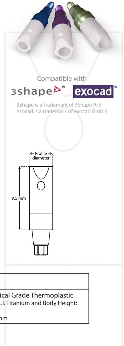
Lower half made of titanium for durability and a temporary, yet secure, connection to the implant
