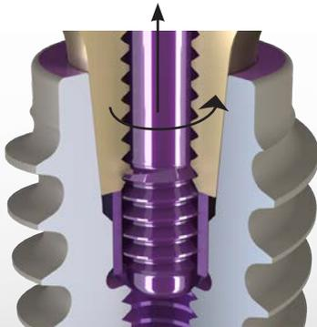
Gently lift up the driver while rotating it counter-clockwise to engage the screw in the internal threads of the abutment.
