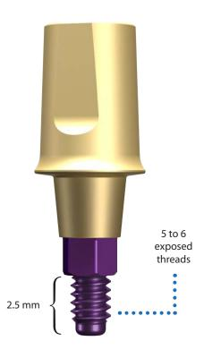
The tip of the abutment screw should protrude approximately 2.6mm (5 to 6 exposed threads).
