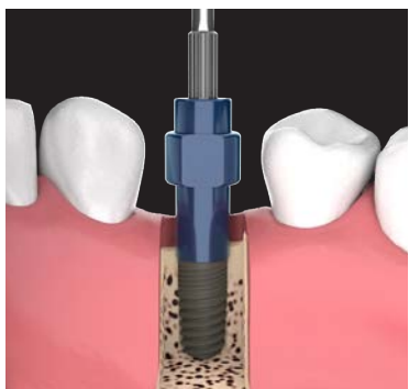
4a.4 Align the appropriate series impression post into the implant. The impression post has a hex on the bottom which will fit into the internal hex in the implant. Finger tighten with .050 hex tool.
