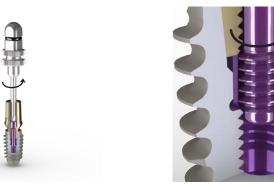
Continue turning the fixation screw counter-clockwise until it disengages the threads of the implant. You will feel it clicking when this happens.
